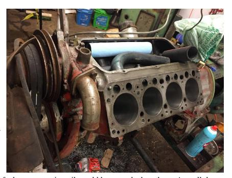
came out. No amount of coca cola, diesel fuel, or penetrating oil would have worked on these. As well the rings were seized to the pistons.
